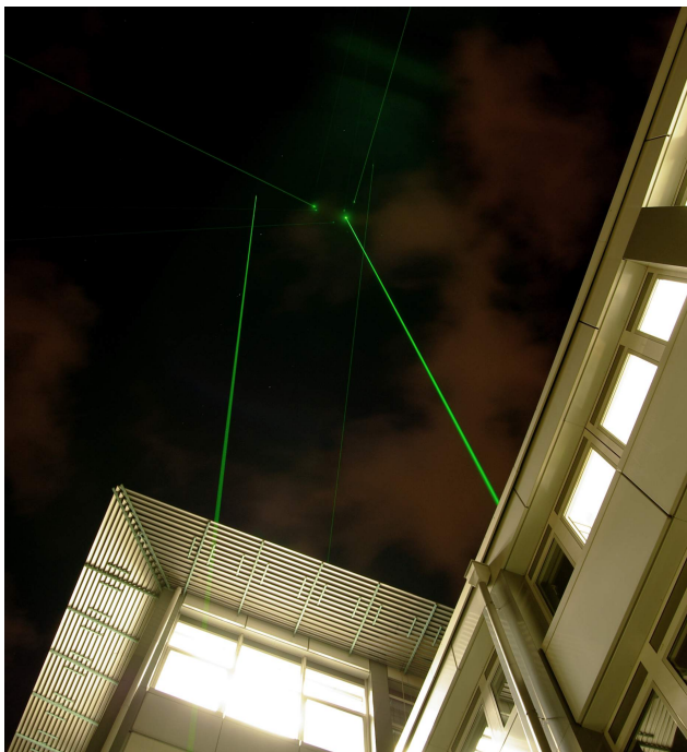
Fig. 2: Measurement of several LIDAR systems at Leibniz Institute for Tropospheric Research Leipzig, Germany. Visible are the building of the IfT and the green laser pulses emitted into the atmosphere by the lidar. Source: IfT
