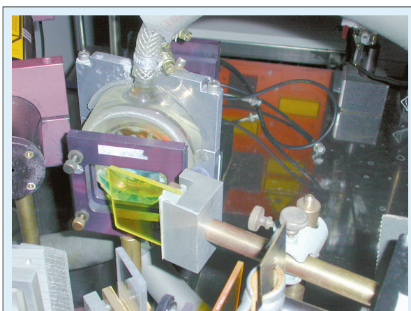
Fig. 7: A laser photolysis-long path laser absorption experiment for the study of nitrate radical kinetics in aqueous solution.
