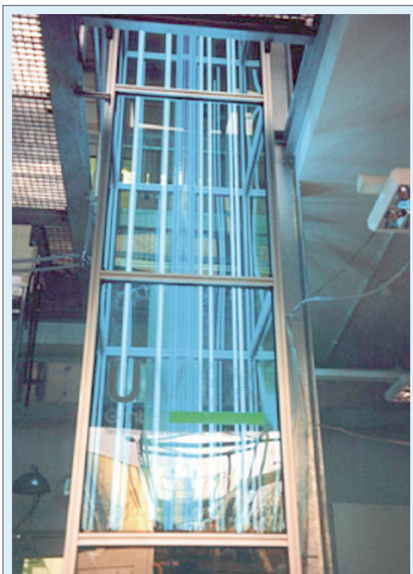
Fig. 6: The IFT laminar flow tube reactor (IFT-LFT).
