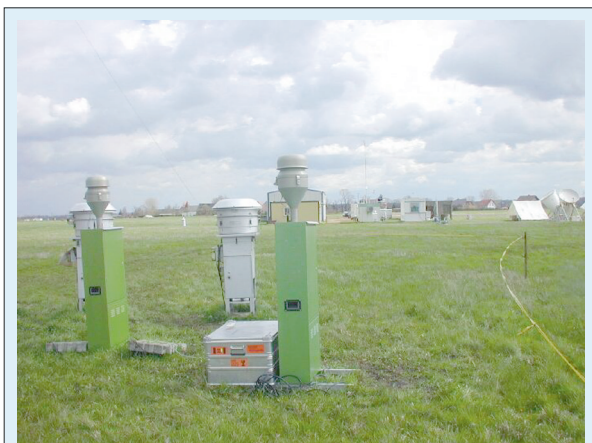
Fig. 2: Particle sampling systems during the INTERCOMP 2000 campaign at the research station Melpitz.
