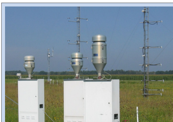
Fig. 1: High volume filter samplers for \text{PM}_{10} , \text{PM}_{2.5} and \text{PM}_1 at Melpitz site.
