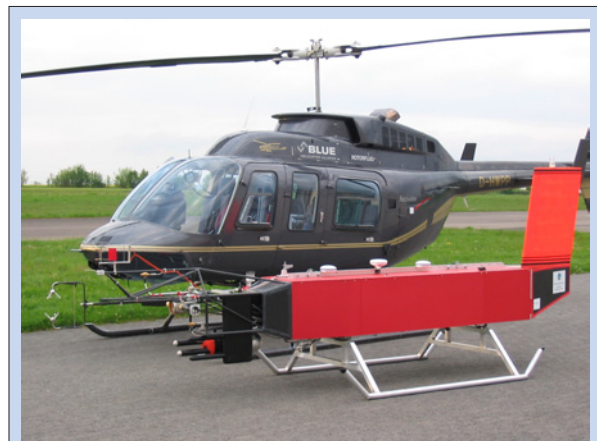
Fig. 1: The new helicopter-borne ACTOS in front of the BELL 206 LR (Long Ranger).
