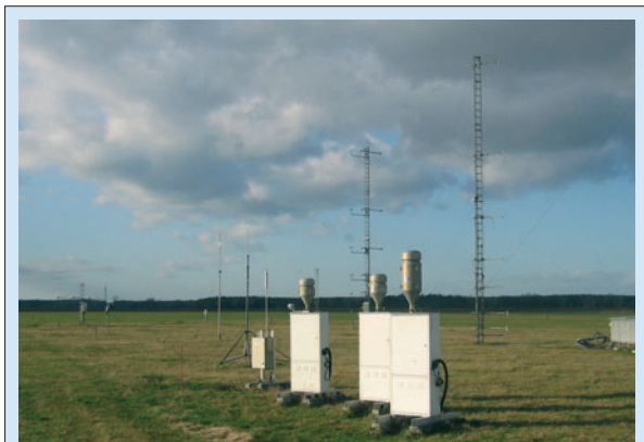
Fig. 1: Measuring field of the IfT research station Melpitz (view towards North). The three DIGITEL High-volume-samplers for PM_{10} , PM_{2.5} and PM_1 are in the foreground.
