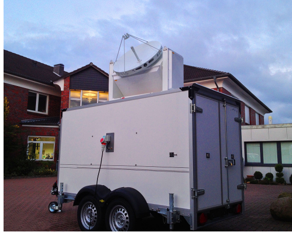
Figure 3.4: The MIRA-35 cloud radar with the scanning unit at METEK GmbH. The photo was provided by METEK GmbH.
