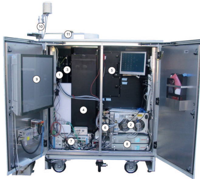
Figure 5.1: The depolarization Raman lidar system Polly XT in its rainproof cabinet. This figure is adopted from Althausen et al. (2009). 1: Laser head, 2: Laser power supply, 3: Beam expander, 4: Receiver telescope, 5: Receiver with seven channels, 6: Power supply, 7: Computer with data acquisition and interface cards, 8: UPS, 9: Air conditioner, 10: Sensor for outdoor temperature and rain, 11: Roof cover.
