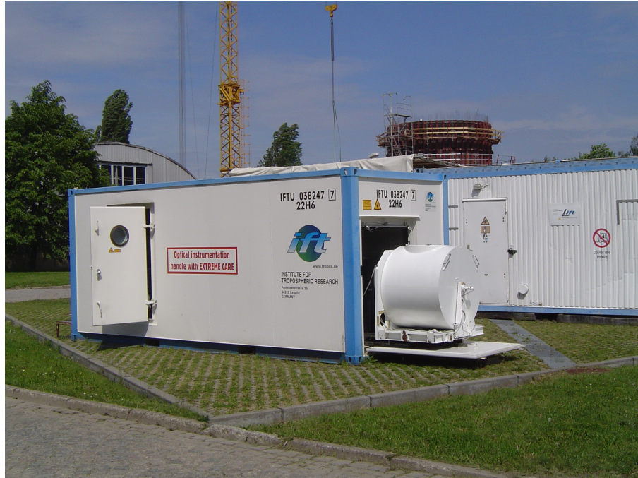
Figure 4.2: Container housing of BERTHA. The deflecting-mirror to deflect the laser pulse into the atmosphere and reflect the incident light to the telescope can be seen on the front right side of the picture (made by D. Althausen).
