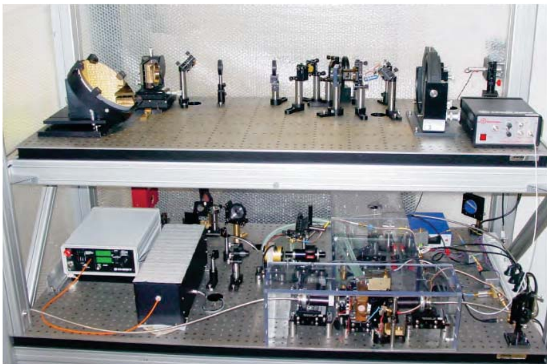
Figure 4.4: Coherent Doppler lidar system deployed in the SAMUM-2 experiment at Praia Airport, Cap Verde. Top: container with its beam-steering unit on top (photograph by J. Fruntke, 2008). Bottom: setup of the optical benches inside.
