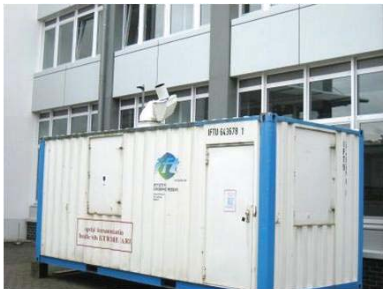
Figure 12: The Doppler lidar WiLi installed in a container.
