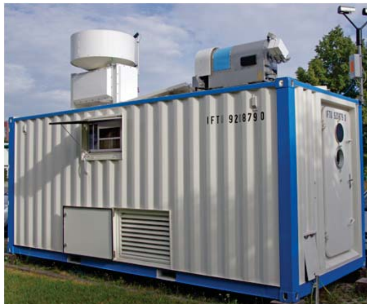
Figure 11: The cloud radar Mira-35 and the microwave radiometer HATPRO installed in a sea container at TROPOS.
