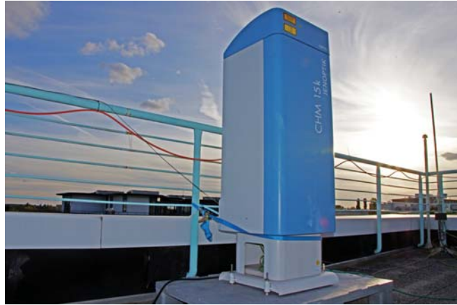
Figure 13: The Jenoptik Ceilometer CHM15kx installed on the roof at TROPOS.
