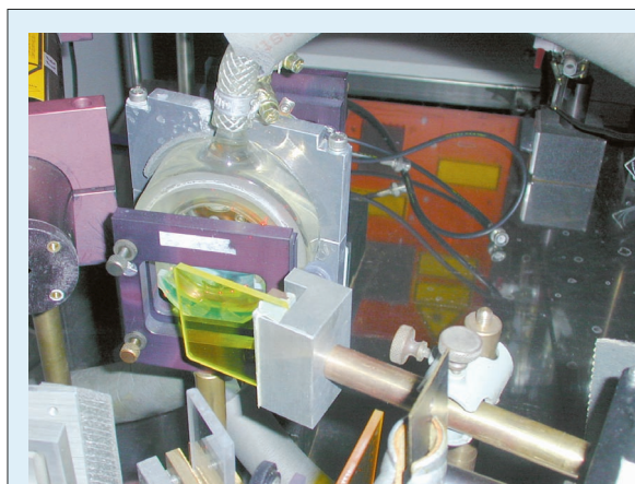
Fig. 7: A laser photolysis-long path laser absorption experiment for the study of nitrate radical kinetics in aqueous solution.
