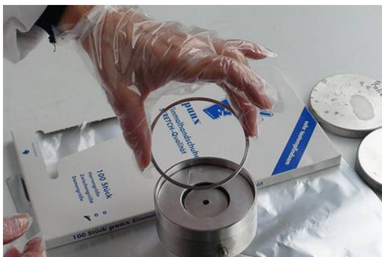
Assembling of a Berner Impactor, Source: TROPOS
