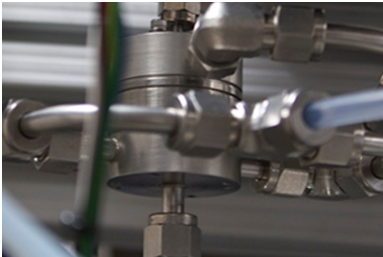
Counterflow Virtual Impactor (CVI), Source: TROPOS
