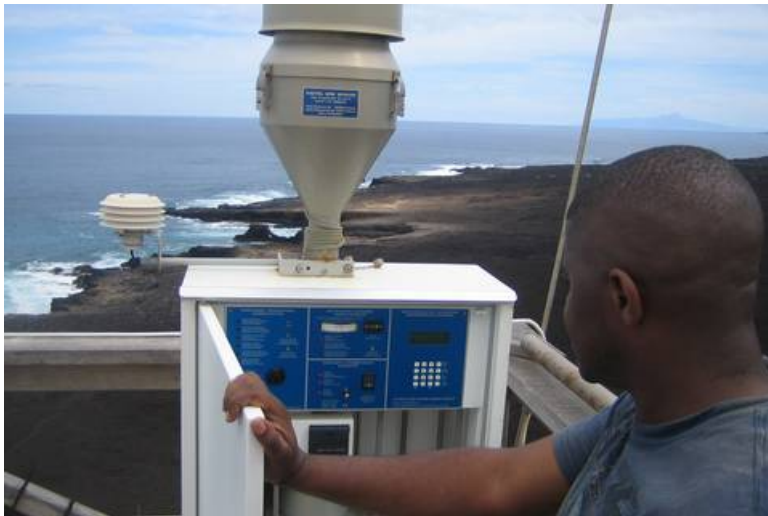
Digital aerosol sampler on the 30m high tower of the Atmospheric Research Station in Sao Vicente, Cape Verde Islands, Source: TROPOS
