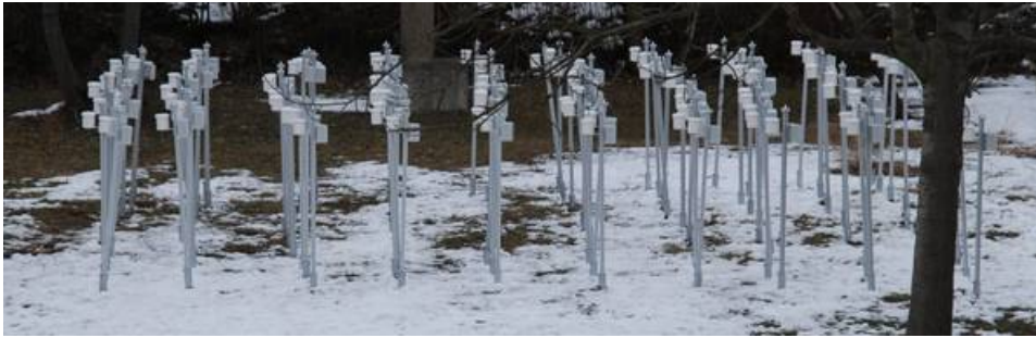
Figure 1: A set of 10 X 10 low-cost ground-based pyranometers arranged for inter-comparison at TROPOS, Leipzig. Source: Bomidi Lakshmi Madhavan/TROPOS
