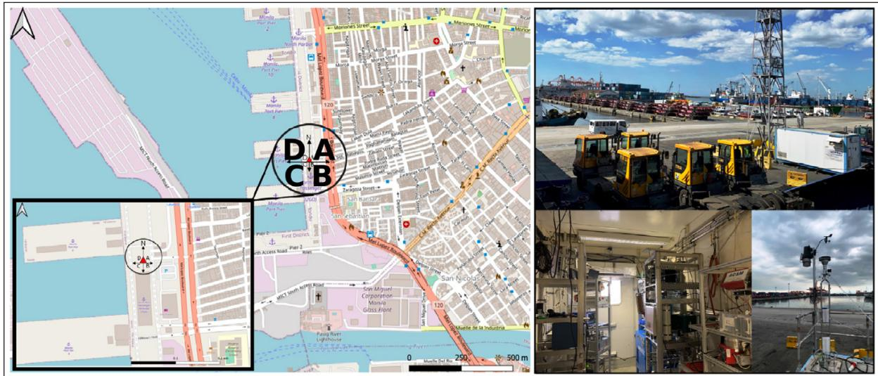
Fig. 3: Measurement site in Manila North Port. The red triangle marks TROPOS measurement container location. Letters A-D indicates wind sector used in data analysis (Sector A - North to Northeast winds; Sector B – Northeast to Southerly winds; Sector C – Southerly to Northwest winds; and Sector D – Northwest to North winds).
