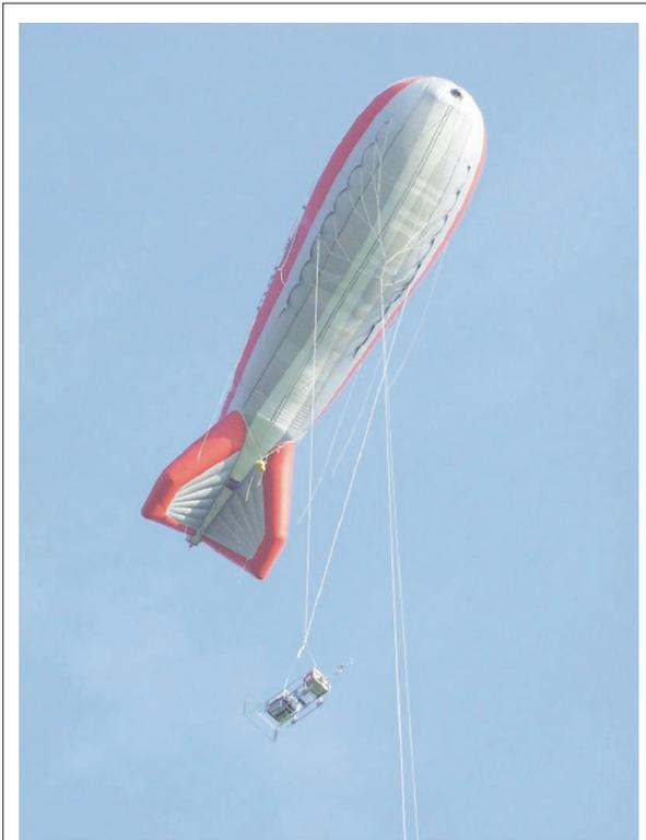
**Fig. 2:** MAPS-Y with the measurement payload.
