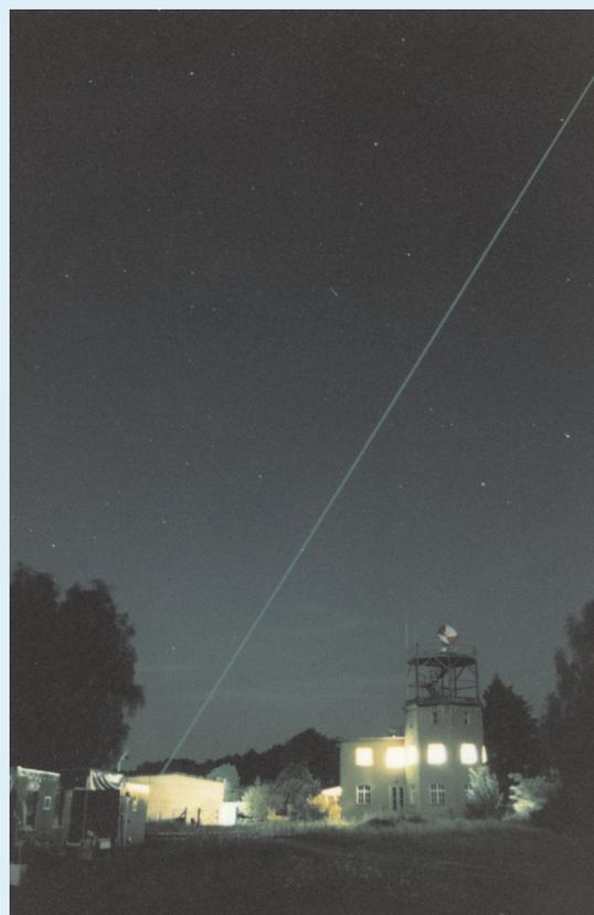
*Fig. 5:* Measurement with the multi-wavelength aerosol LIDAR during a field campaign.
