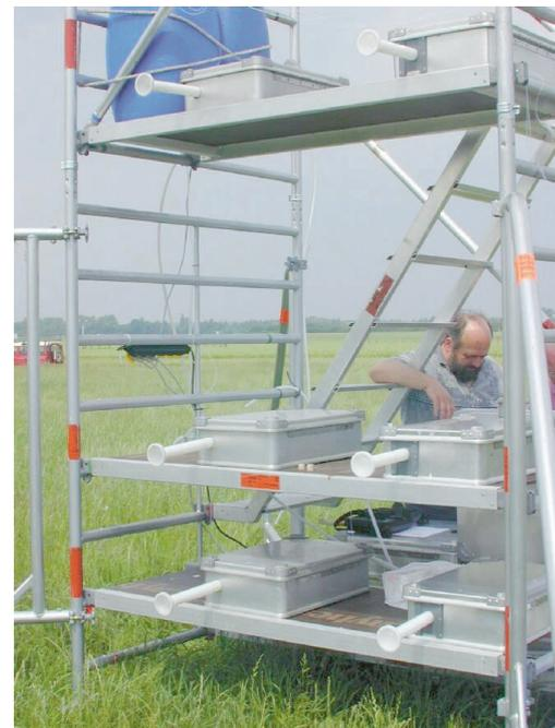
**Fig. 2:** Two gradient systems (AMANDA), both for  $\text{NH}_3$  measurements at three levels above ground, side by side during an intercomparison experiment in summer 2000 at the Bundesanstalt für Landwirtschaft, Braunschweig.
