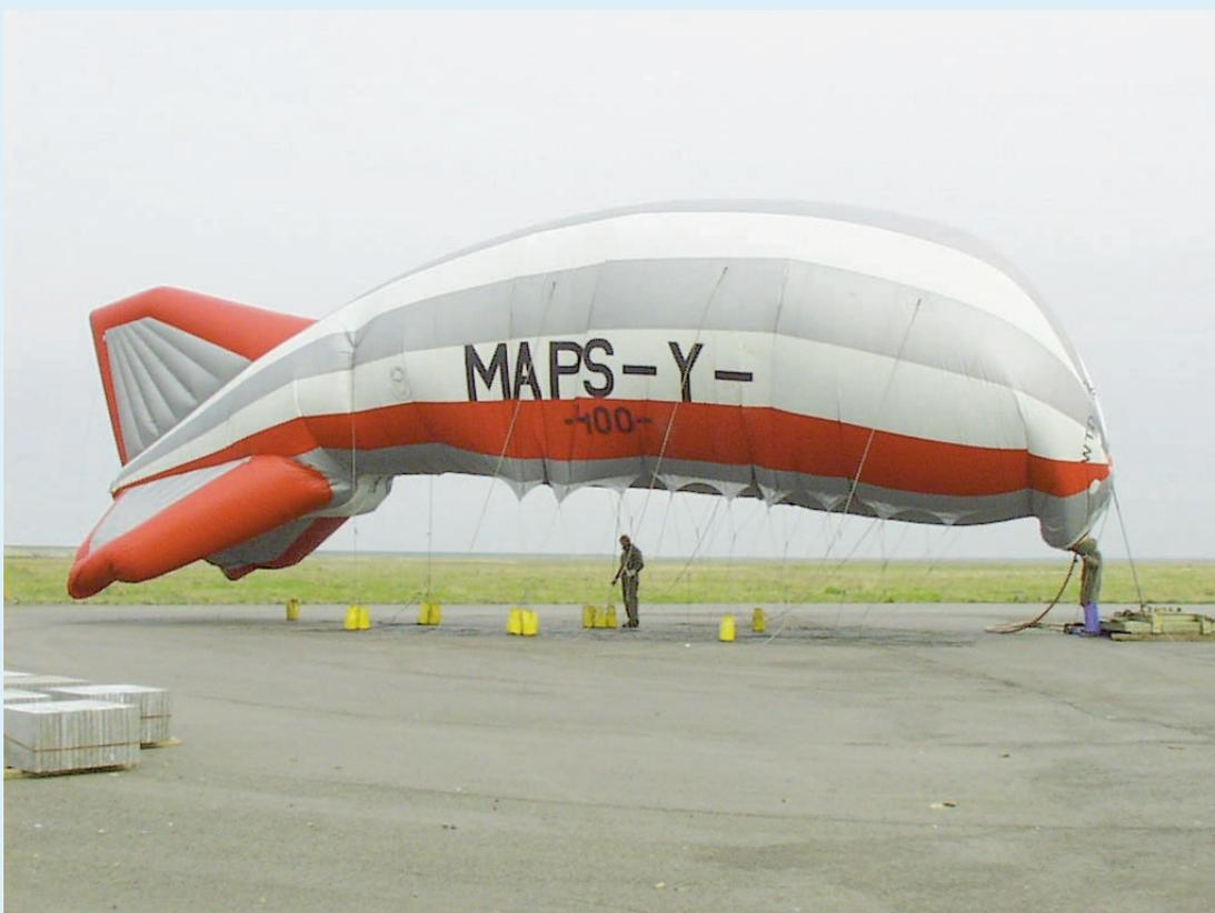
**Fig. 1:** MAPS-Y is filling up with hydrogen before start.
