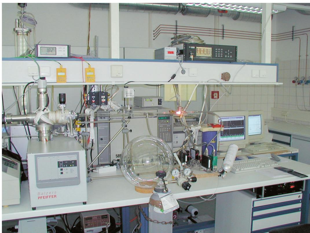
Fig. 1: Experimental set-up for studies of the reaction of OH radicals with aromatics.
