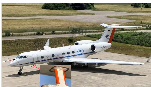
Fig. 1: The German research aircraft HALO with inlets and wing probes in the CIRRUS-HL configuration. The position of the HALO-CVI as the only inlet at the lower fuselage is marked by the red circle and its construction shown in the enlargement.
