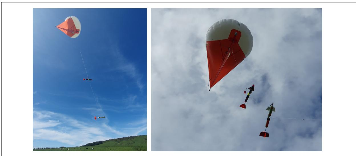
Fig. 4: Helikite carrying a radio sonde of NIWA and the two TROPOS sondes.
