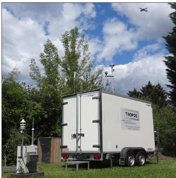
Fig. 1: The TROPOS trailer station at Eichwalde primary school under the BER approach path.
