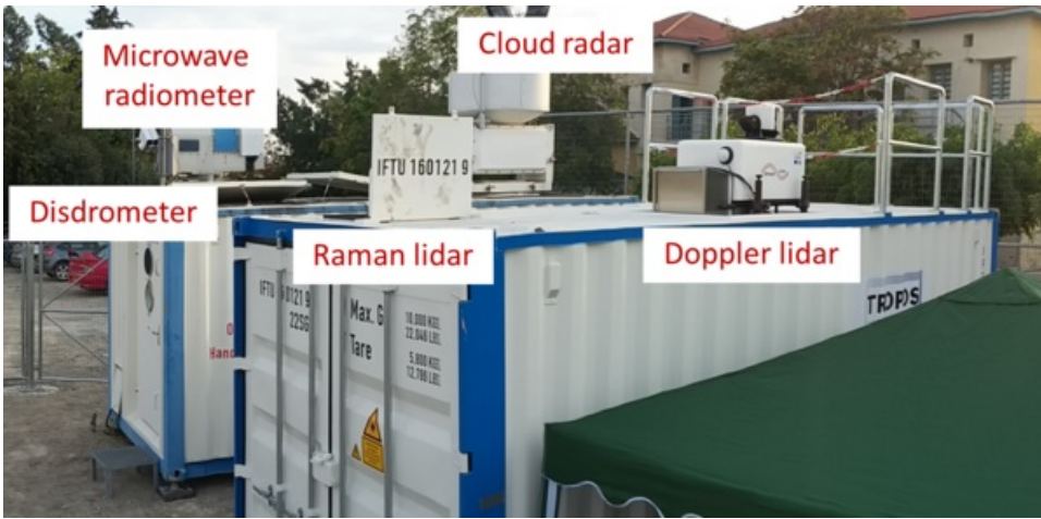
Fig. 2: The measurement systems of LACROS. Different measurement systems are used to measure aerosols (Raman lidar), cloud particles (cloud radar), air motions (Doppler lidar), rain (disdrometer) and water vapor (microwave radiometer).
